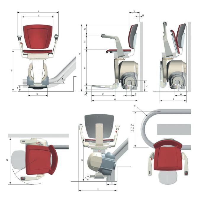
This datasheet is intended to be used for reference only. All dimensions shown from the wall will be affected by any additional obstructions and are subject to a full site survey. Measurements are in millimetres. No rights can be obtained from this datasheet.
