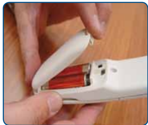
Fig. 4.1: Changing the batteries of the call and send stations.
