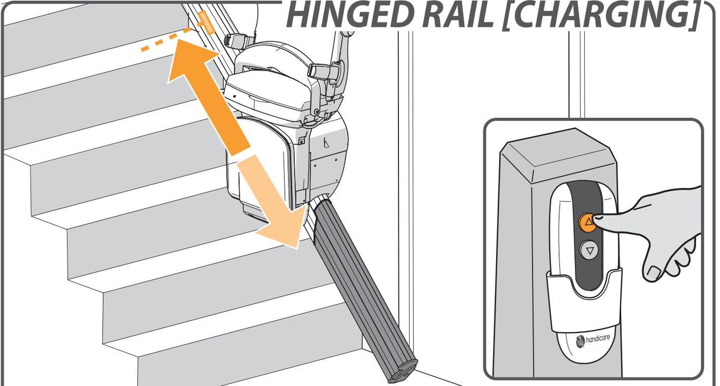
Do not leave the lift on the hinged rail after use. Use the remote control to move the lift to a charge point and recharge the batteries. The first stopping point is a charge point.
