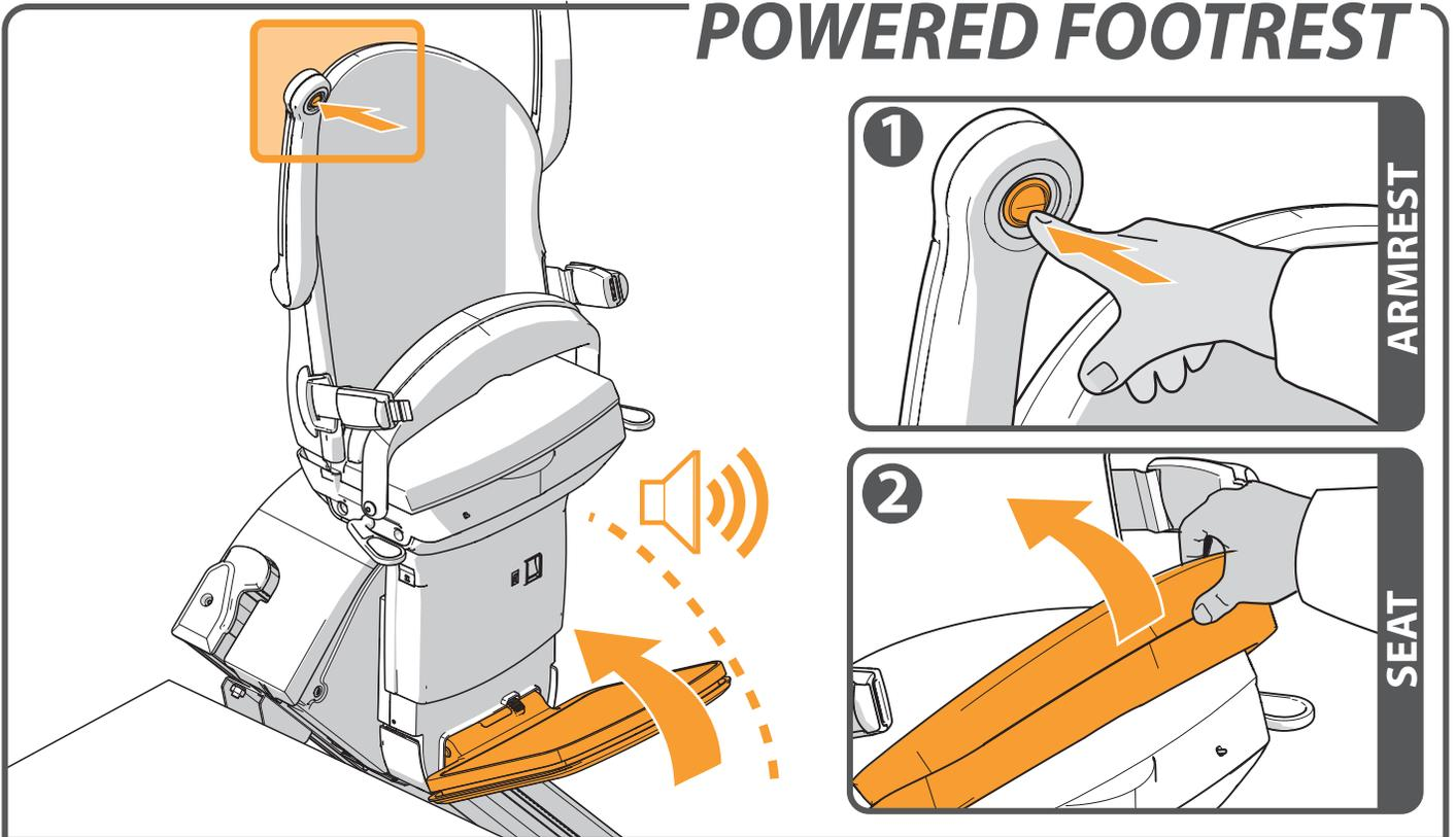
To operate a POWERED FOOTREST move the switch under the armrest[1] or fold up the seat[2]. The stairlift should beep whilst folding the footrest. Always ensure the footplate is in the down position during travel.
