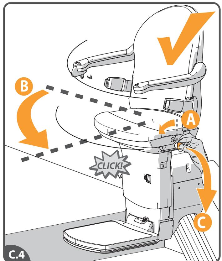
[C.1] If the power swivel is not functioning it can be swivelled manually. Do this only in an emergency. [C.2] Insert a coin in the button on the side of the seat. [C.3] Swivel the seat manually. [C.4] The seat must be returned to the start position. Remove the coin. Do this before you use the lift again.
