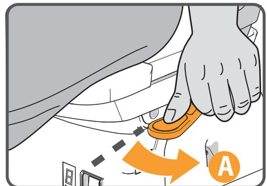
The lift stops automatically at the end of the rail. You should now swivel the seat manually, making it easier to get on and off. To do this, push down the lever{A}. Swivel the seat until you hear a 'click'. The seat is now in the correct position{B}.
