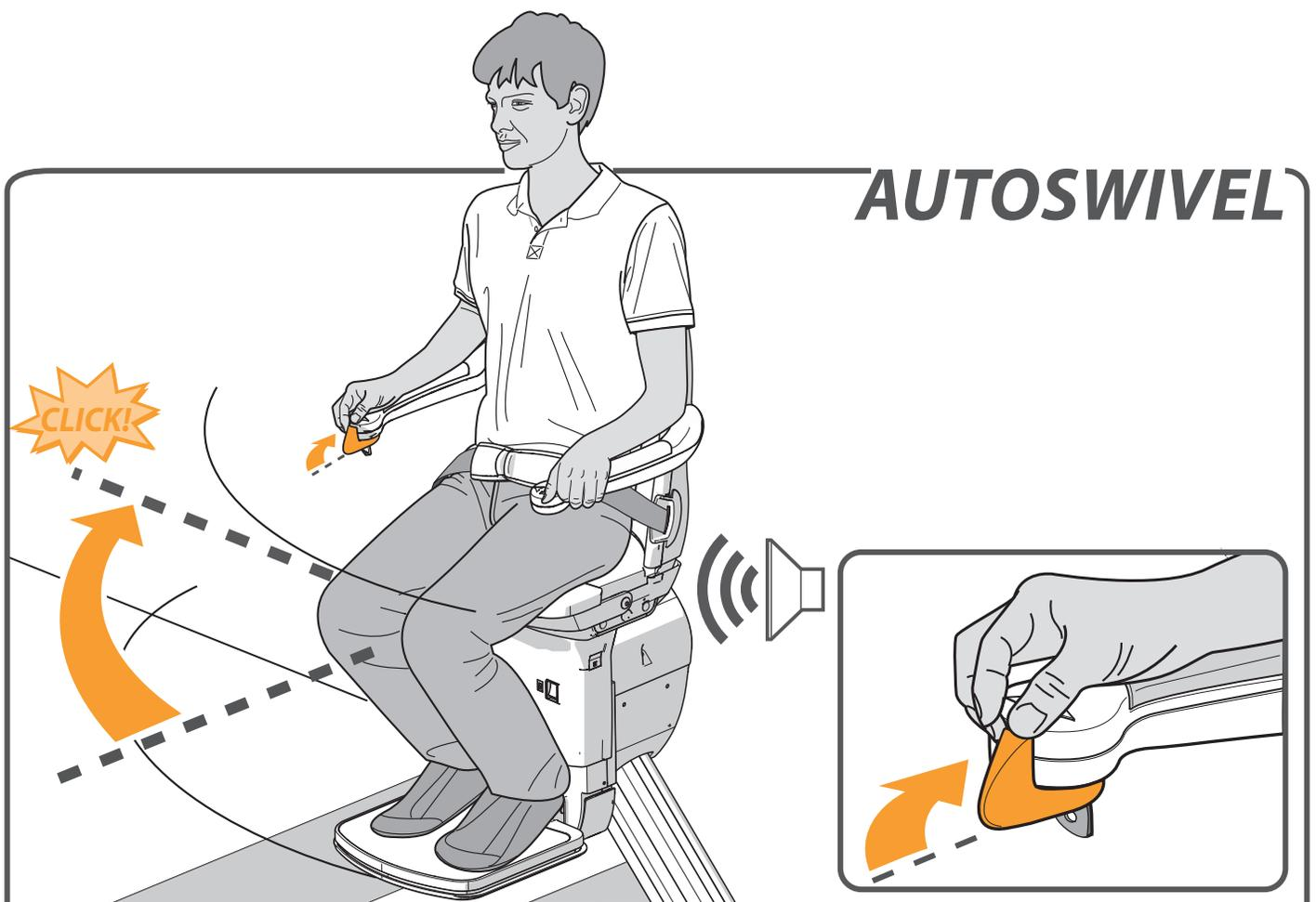
The AUTOMATIC SWIVEL SEAT option lets you swivel the seat automatically to face the direction you are going to walk. To do this, push and hold the joystick in the direction of travel.
