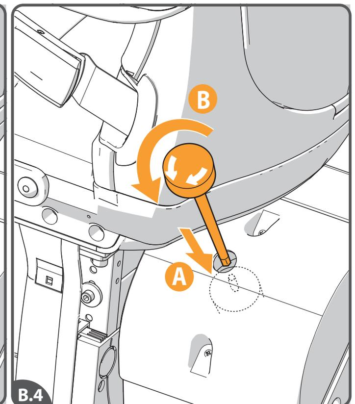
[B.1] When the stairlift stops unexpectedly and no longer moves any further, the hand winder can be used to move the lift to a charging point. [B.2] Turn off the lift. [B.3] Remove the cap from the unit with a screwdriver. [B.4] Turn the hand winder as indicated on the winder. Then wind the lift in the required direction.
