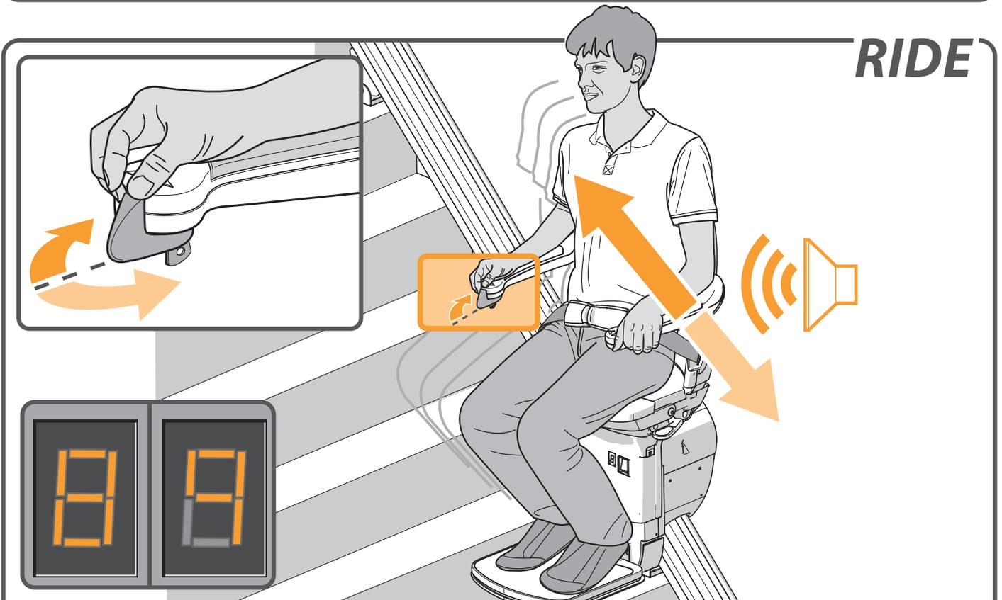
Move and hold the joystick in the desired direction of travel. The display shows a “8/9”, the lift will beep 3 times and start slowly after 1 second. When changing the direction of travel the delay will be 3 seconds.
